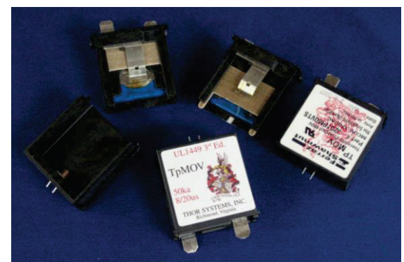
Thermally Protected Metal Oxide Varistor (TpMOV) "Fail-Safe Device"
